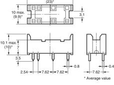
PCB Mounting Holes (BOTTOM VIEW)
